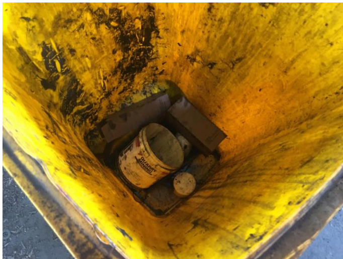
Plate 4.3 Inappropriate waste disposal, with general waste in an oil rags bin
